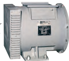
Brushless, self-regulated design produces 460 volts, 18kVA, 15kW @ 0.8 pf.
