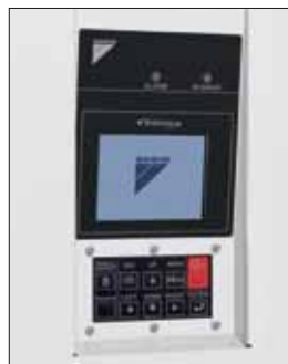
Features a large (5.7-inch), easy-to-see, backlight LCD
