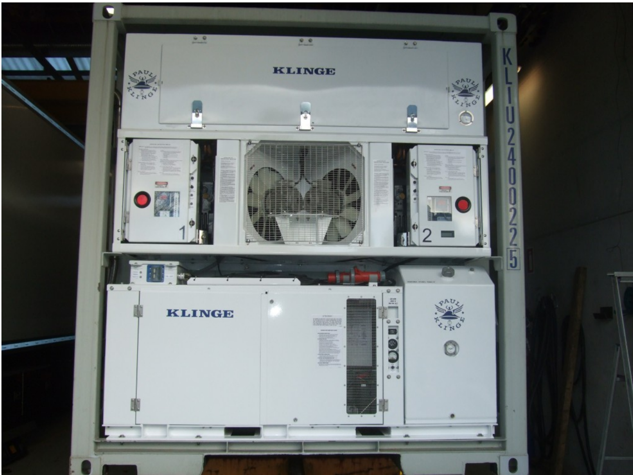
Dual Refrigerated Container (two full capacity reefers) with Integral Generator Set
