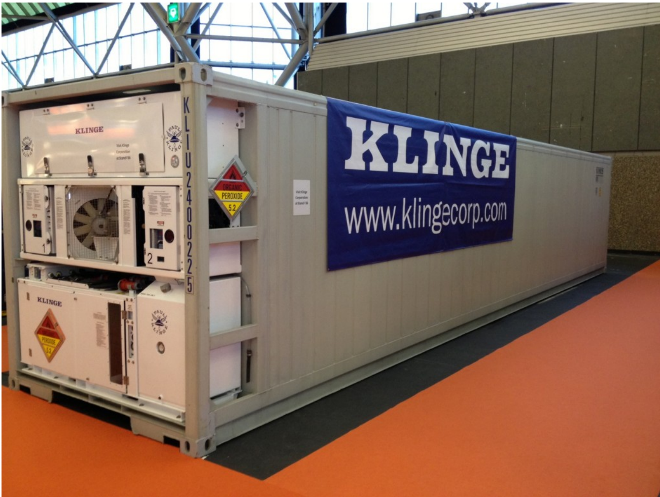
Dual Refrigerated Container (Two complete and separate refrigeration systems) with Integral Generator Set
