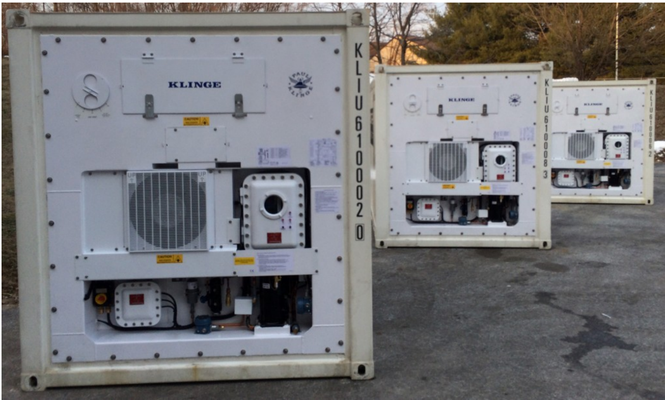
Explosion-Proof Refrigerated Container (Atex compliant reefer & container certified to DNV 2.7-1
